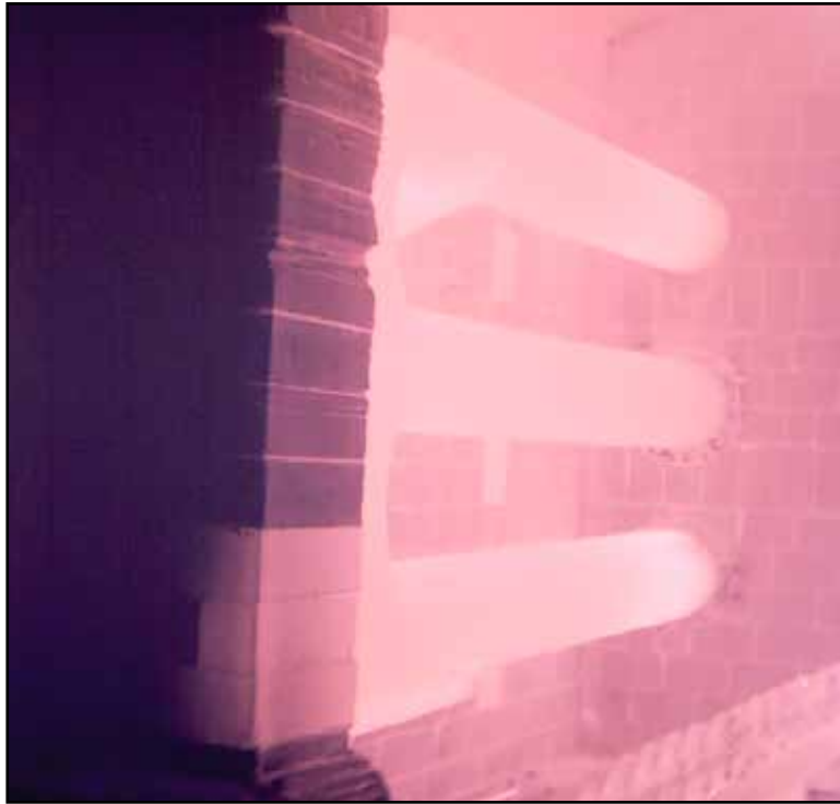
RA 602 CA Tubes - Taken after 1 year in service at Euclid Heat Treat
